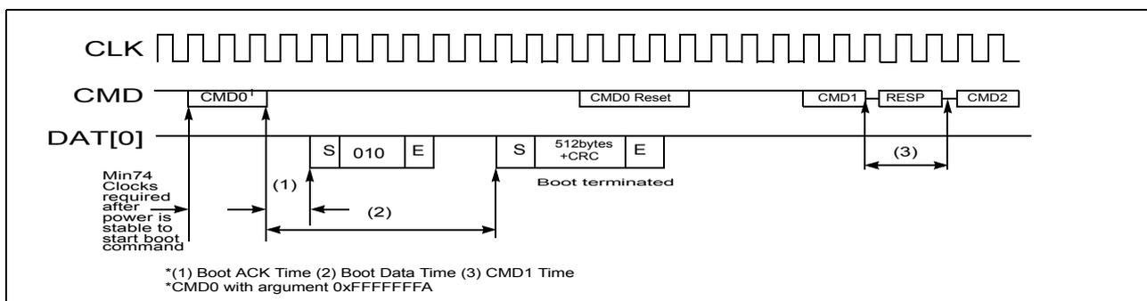
Figure 5. embedded MultiMediaCard state diagram (alternative boot mode)
